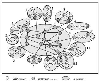
A topology generated using transit-stub model, except domain 0 in the middle borrows from the AT&T Worldnet IP backbone
