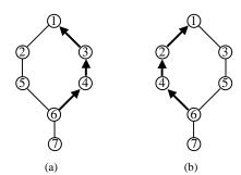
Figure 2: An example topology with two equal-cost paths
