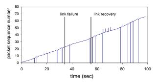
Vertical bars below the graph mark bad packets that are detected and dropped; vertical bars above the graph mark good packets that are incorrectly dropped.
