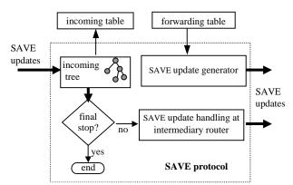
Figure 3: The architecture of the SAVE protocol
