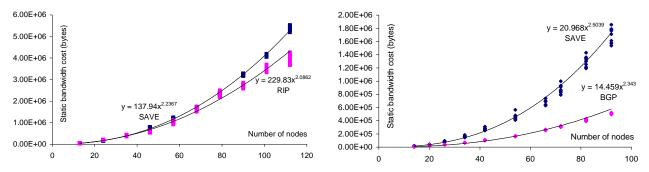
Figure 14: Static bandwidth cost comparison between SAVE and RIP Figure 15: Static bandwidth cost comparison between SAVE and BGP
