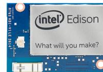
4. If the Edison reboots as soon as you connect a servo, your system is not supplied with enough power. Make sure to use a powered USB hub or an external power supply that can supply enough power.
