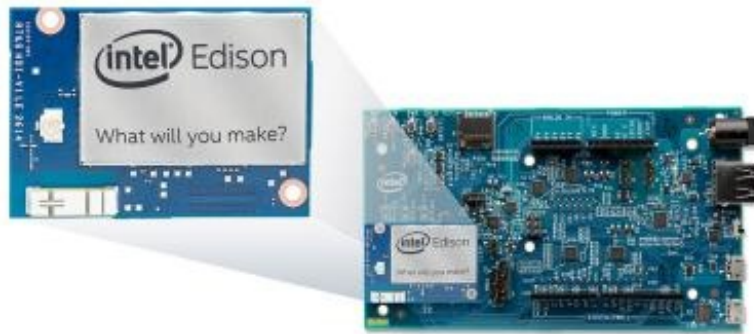
Figure 1. Intel Edison Compute Module attached to Edison Board for Arduino
