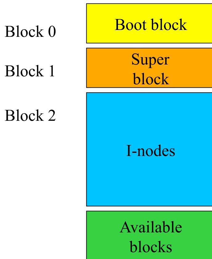
Block size and number of I-nodes are specified in super block
