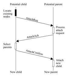
Fig. 1. Three-way-handshake protocol.
